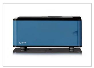
For repeateble results the product is placed into a sample drawer, which can be comfortably opened and closed. Magnets keep the drawer to hold the micro-gloss in place and allow non-contact measurements of your products in a completely shielded compartment.
