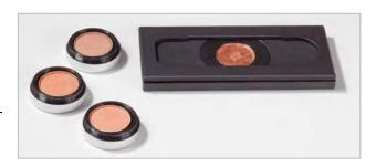
For repeatable results the product is pressed or pured into a sample cup. During sample preparation of pressed powders, it is important to always maintain the same plunger pressure as well as the same plunger tissue. It is recommended to use a fine-woven fabric to create a smooth, non-textured surface. The holder is equipped with a mask onto which the micro-gloss is placed for non-contact measurements.
